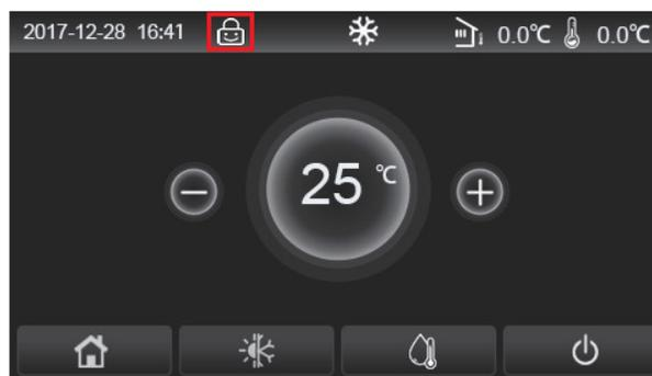
In this case, the control panel is locked and any touch operation does not work. By touching
