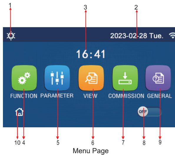
Above the menu, the corresponding icon will be displayed based on the mode and status of the control panel.
