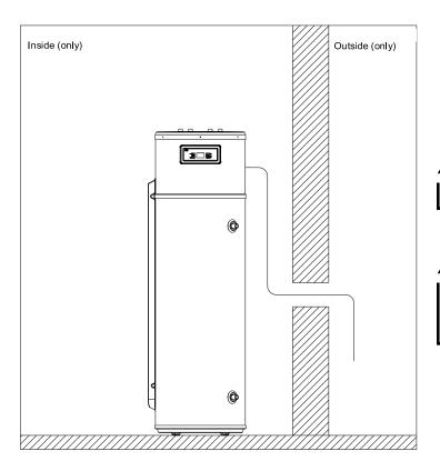
The Pilot's pressure-relief valve drainage pipe must be properly secured until the outside of the building without any pinching zone.
