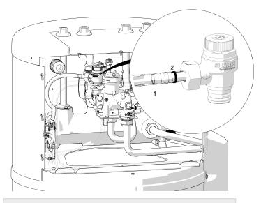
The EPDM pipe must be pushed to the end of the safety valve barb tip and held with a hose clamp.
