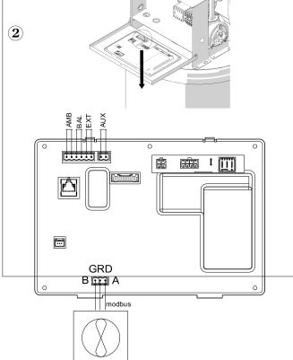
ModBus: Connection to the heat pump
