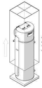
On reception of the pilot, check the state of the cardboard packaging as well as the general state of the product. Remove cardboard box by pulling it up.
