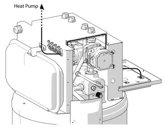
Plan for the appropriate length of cable between the pilot and the heat pump. Do not hesitate to cut the cable to the appropriate length to **AVOID LOOPS**.
